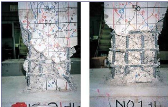
A) Hoops with OS Clip joints B) Hoops with flare-welding splices
