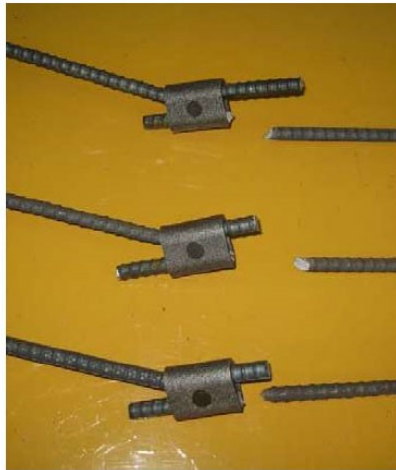
Specimens after tensile test
