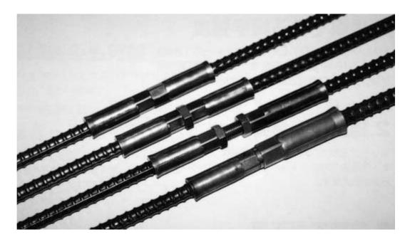
C-S-Joint Method is a mechanical joint method setting the sleeve to both ends of the connecting Re-Bar, splicing one side of sleeve and connecting the other side of sleeve with intermediate bolt.
