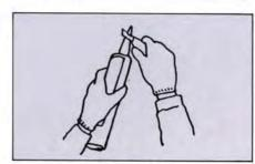
Cut nozzle at area for desired dimention. Puncture damp-proofing film. Remove rear cap.
