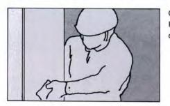
Clean the surface. Remove the dirt, oil and scale.
