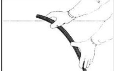
Remove the release paper from MC-2005T and press the product very firmly onto the Butyl tape. Check for any gaps between the product and the substrate. If gaps are present, fill the gaps using ADEKA P-201 applied to the side of the strip. Use ADEKA P-201 on concrete joints and on side-by -side splice joints as usual. You can place concrete immediately, no waiting for curing time.
